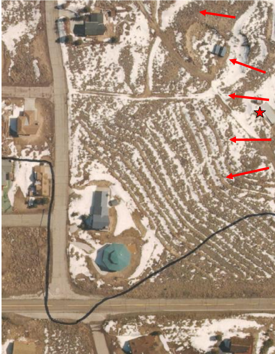
Figure 4. Aerial photograph water tank with avalanche flow directions as red arrows. The water tank is the rectangular building to the right of the star. Historic avalanche runout boundaries taken from Mears, 1989, figure 2-4.
